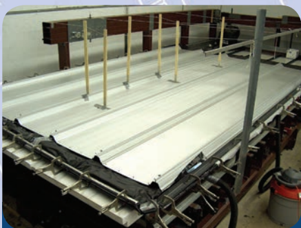
ASTM E 1592 test set up before load applied
